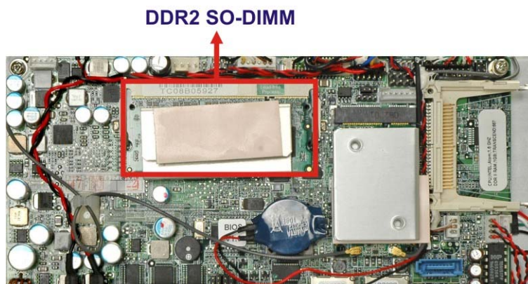
Figure 3-4: AFL-08B-N270 SO-DIMM Socket Location
