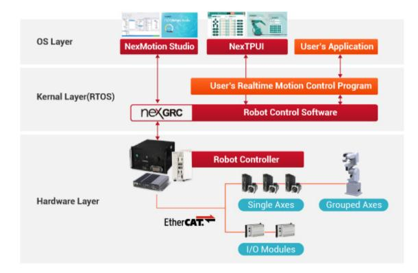
NexCOBOT GRC provides the essential components for easier setup of EtherCAT devices and modules, enhancing user experience through its intuitive NexTPUI user interface, putting complete control in users' hands through the powerful yet familiar programming experience of NRPL, and allowing for customization through the NexMotion Studio API.
